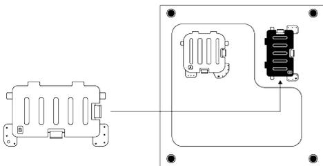
Rest the tabs of Cover B against the lower panel. Complete the assembly by rotating the cover.
