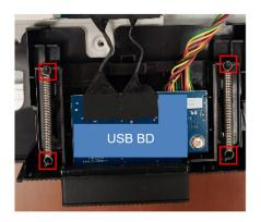
S15 Unlock 4 screws to disassemble USB BD module from Middle Frame
