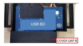
S25 Unlock 2 screws to disassemble USB
