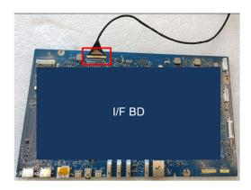
Unplug "SPS BD to I/F BD wire" and "WIRE AC+3/3P" from SPS BD, then, disassemble SPS BD from Main SHD
