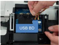
S17 Unplug 2 "LED Driver BD to Panel wires" from LED Driver BD
