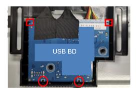
S27 Tear off 2 tapes from USB BD and USB wires as picture shown
